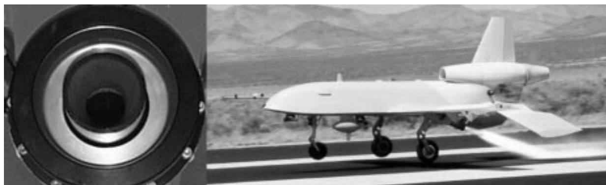
Left: RATO pack with AeroPack RA98 Motor Retainer and AeroTech™ motor. Right: Prowler UAV in STO launch using RATO pack with AeroTech™ M2500 motor and Aero Pack RA98 Motor Retainer. Acronyms: RATO = Rocket Assist Take Off, UAV = Unmanned Aerial Vehicle, STO = Short Take Off. Photos courtesy of General Atomics Aeronautical Systems Division
